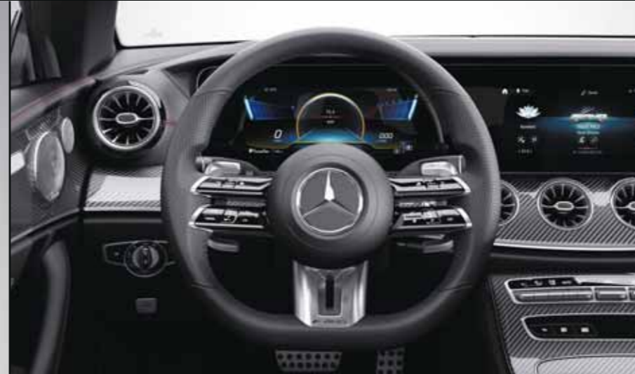
L6J - AMG Performance steering wheel in Nappa leather with touch control panels, galvanised shift paddles, flattened bottom section and "AMG" lettering
