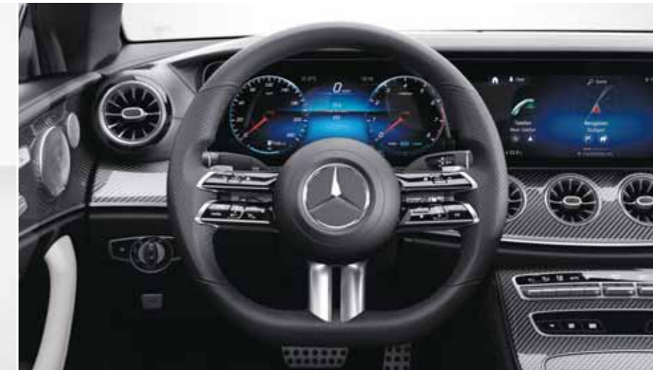
L5C - Multifunctions sports steering wheel in Nappa leather with touch control panels, galvanised shift paddles and flattened bottom section
