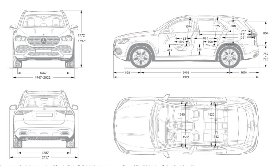
¹ At minimum to maximum height with steel suspension. All figures in millimetres. The illustrated dimensions are mean values. They are valid for vehicles in basic specification and in unladen condition.
